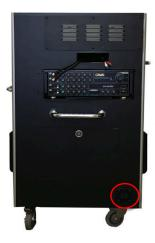
3. Use the key to open the bill acceptor compartment on the right side and the speaker compartment on the back side of the kiosk.
