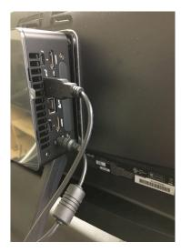
3. Next using an enclosed short HDMI cable, connect the touch screen monitor to the karaoke player as shown.
