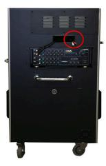
Connecting additional speakers directly onto the CA-242RA amplifier is not recommended as it will more likely cause blow-out of amplifier or the speakers when playing aloud.
