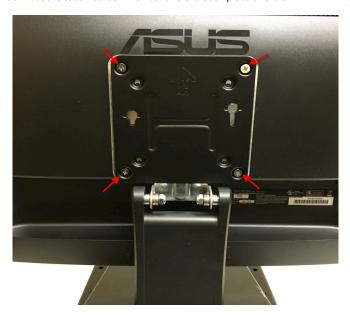
Be sure the monitor stand is in-between the touch screen monitor and the back plate of the JB-199 mini II. Also be sure the back plate of the JB-199 mini II is correctly oriented, as shown in the picture.
