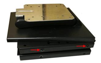
User  $4 \times 10^{-2}$  x black screws as shown in the picture (and in the opposite side) to connect. Be sure to attach the two parts in the correct orientation.
