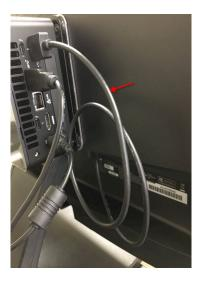
Using an enclosed short USB cable, connect the USB-B end of the cable to the touch screen monitor and USB-A end of the cable to the karaoke player.
