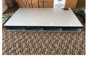
Next attach the enclosed rackears to the NAS server. There are only 2 front rackears.
