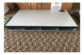
Next attach the enclosed rackears to the NAS server. There are only 2 front rackears.
